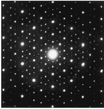
Fig. 1. Selected area electron diffraction pattern taken with an incident beam along a five-fold axis for an icosahedral Zn_{50}Mg_{42}Y_8 alloys before hydrogenation.
